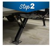
**TO EXTEND:** Press the "EXT" buttons until each leg reaches the ground. The sound of the motor will change pitch as the legs begin to take weight. Adjust each side independently for desired stability.
