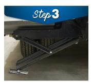
**TO RETRACT:** Press the "RET" buttons simultaneously until each leg is fully retracted.
